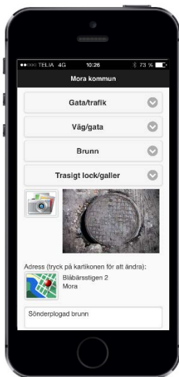
Infracontrol Online collects information about faults from residents and technical installations so that they can be sent to the right person for action. When the fault has been remedied, it’s reported to the municipality concerned, which uses the information and take proactive measures to prevent similar problems from occurring again.
