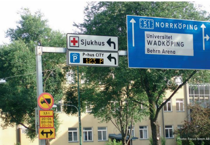
The City of Örebro now has a parking guidance system that improves traffic flow and the town's urban environment. The system, which makes parking easier, was inaugurated on January 16, 2009. The system is based on Infracontrol Online and comprises around 40 dynamic parking signs that point the way to vacant spaces in 6 different parking facilities.
